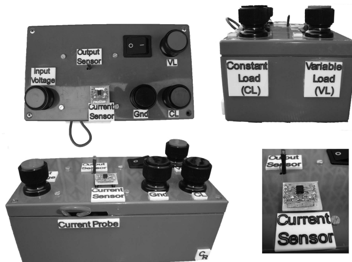
Figure 3-23: Different views of the current sensor test box.
