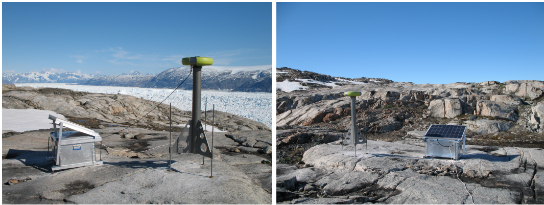
Figure A.2: Pictures of a GPS reference static station deployed at Helheim on the glacier margins during summer 2006.
