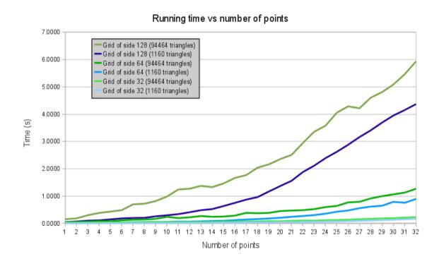
Figure 5.14: Running times for the computation of the 3D good-visibility map when the number of viewpoints and grid size increase. These plots compare the times for the same scene using 1000 and 100000 triangles to represent it, respectively.
