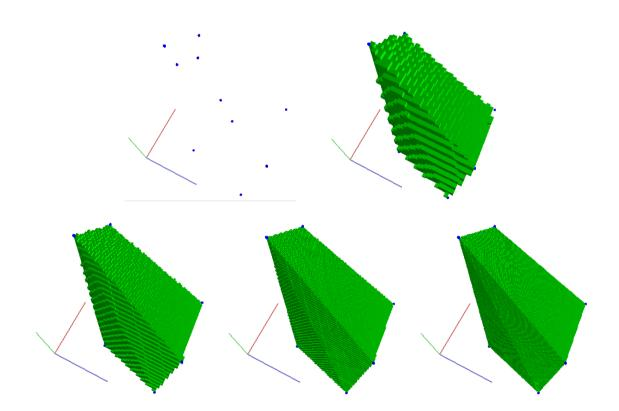
Figure 5.2: The top-left image shows how the 10 points in the space are placed. The other pictures show the  $C_1(V)$  discretized in a space of side 32, 64, 128 and 256 voxels, respectively.
