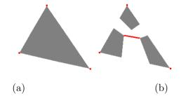
Figure 4.2: (a) Good-visibility map of a set of three points. (b) When an obstacle is added the 1 good-visibility region becomes smaller and disconnected in some polygons.
