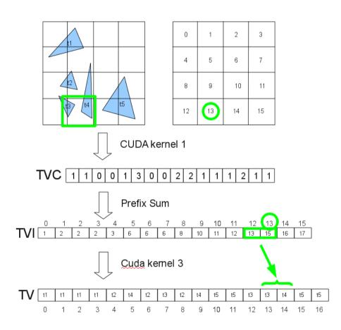
Figure 3.18: The scheme of the voxelization of the triangles. The upper images show the obstacles, the voxels forming the uniform grid and the index of every voxel. The green squares indicate the voxel we are interested in and where we can find the triangles it intersects. The green circles indicate the index of the voxel of interest.
