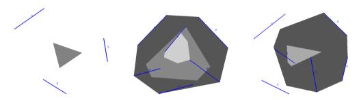
Figure 4.21: From left to right images show the computation of the depth map from a set of view segments using strong visibility (S), weak visibility (W) and a mix of them, respectively.
