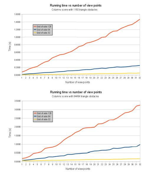
Figure 3.23: The images show the running time for the 3D visibility computation using the explained CUDA method. Times on the top image are taken from a scene with 1000 triangles while times on the bottom image are based on the same scene with 100000 triangles.
