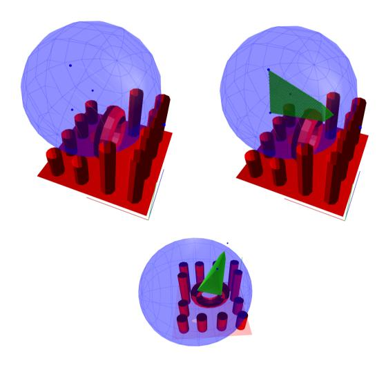
Figure 5.15: The top-left image shows the scene from which the good-visibility map is computed. Notice that one of the viewpoints uses restricted visibility. The result is shown using different points of view in the other images.
