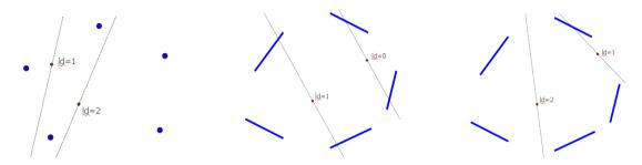
Figure 4.19: Left image shows how the location depth works when V is a set of viewpoints. In the middle and right images, strong and weak location depth can be seen respectively, when V is a set of view segments.
