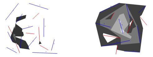
Figure 4.22: The images show the good-visibility map from a set of 11 view segments with strong visibility and from a set of 8 view segments with weak visibility, respectively.
