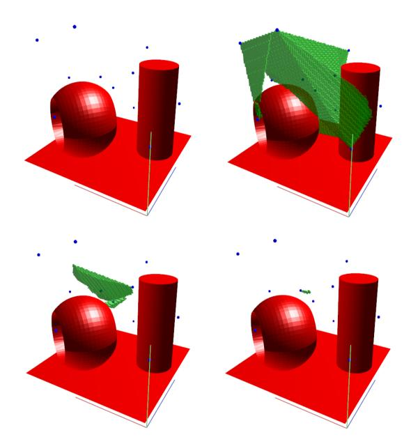
Figure 5.13: The top-left image contains the scene from which the good-visibility map is computed. The other three images show, one by one the good-visibility regions  $gvr_{V,S}(1)$ ,  $gvr_{V,S}(2)$  and  $gvr_{V,S}(3)$ , respectively. Notice that a slightly transparent effect is applied to the visualization.
