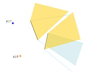
Figure 4.11: Shadow regions with signal crossing segment obstacles. Point p has sufficient power to cross one segment obstacle.
