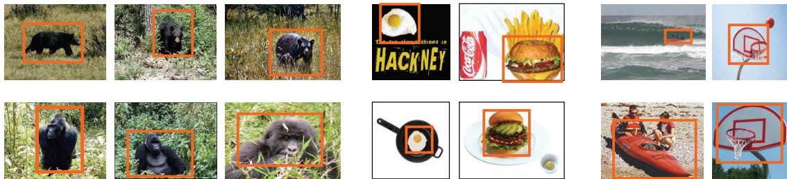
Figure 6.17: The red patch represents the part of the image which contains the objects. Using only this patch to compute the pyramid descriptor will provide a better representation for the objects without taking the background into account. In this case translations and scale variances can be avoided.
