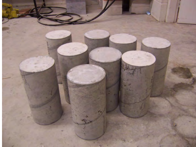
Figure 5.10: Concrete control samples used to obtain concrete mechanical properties.
