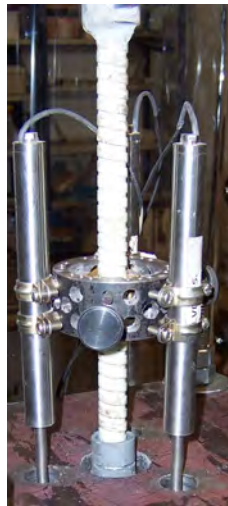
Figure 3.7: LVDTs at the top face of the cube.
