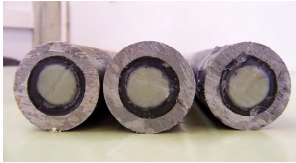
Figure 5.2: Detail of the rebar alignment with steel housing.
