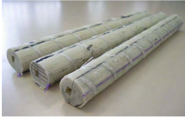
Figure 5.9: 200mm long samples to measure glued rebar geometrical properties.
