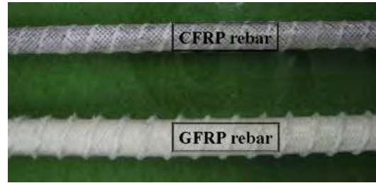
Figure 2.22: FRP rebars used in [41].
