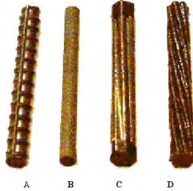
Figure 2.14: Carbon fiber reinforced polymer bar types used in [30].
