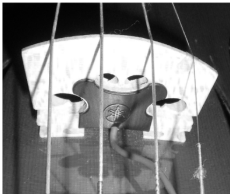
Figure 2.2: Detail of the Yamaha © VNP1 bridge piezoelectric pickup mounted on the violin.
