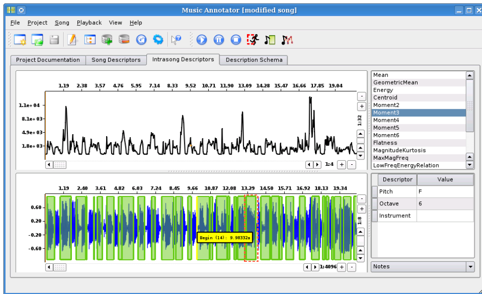
Figure 6.4: Editing low-level descriptors and segments with the CLAM Annotator. This tool provides ready-to-use descriptors such as chord extraction and can also be used to launch custom algorithms
