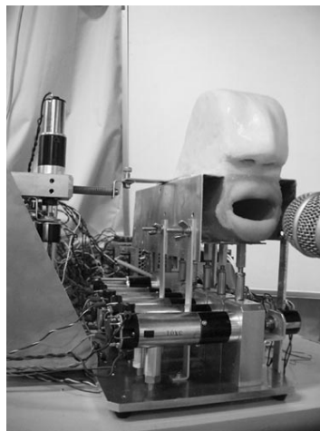
Figure 49: Picture of Sawada's mechanical voice system
