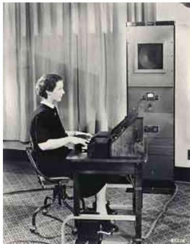
Figure 50: According to Science News Letter, of January 14 1939, "The young lady striking keys is creating a man-like voice. This new synthetic orator will "lecture" with his "electrical accent" at the New York and San Francisco world fairs. It is a compact machine resting on a small table, plus as many loudspeakers as are necessary to reach the audience. VODER, THE MACHINE THAT TALKS. No recording of any kind is used in this latest addition to the anatomy of the Mechanical Man. A girl at a keyboard controlling varying electrical currents does the trick. A pedal operated by her right foot enables the operator to make voice inflection, and synthesized speech is heard from a loudspeaker."
