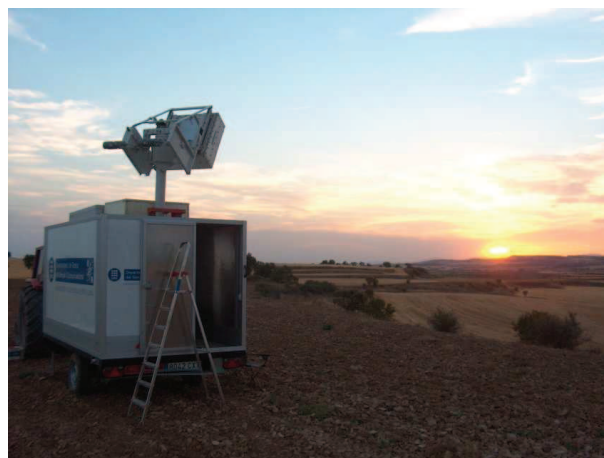
Fig. 9.2: The LAURA radiometer at the T-REX 2006 experiment site during the Sun measurements.
