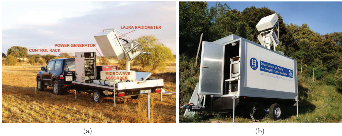
Fig. 4.3: Trailer containing the LAURA radiometer, its control rack, a power generator, and the microwave absorber for hot load calibrations. (a) First configuration and (b) present configuration.
