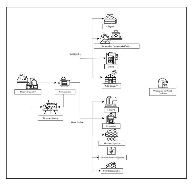
Figure 4. Main manure treatment technologies to produce organic and BBF. \*The same technologies can be applied to both manure or digested manure, being the digestate more stable and releasing less emissions. \*\*Discussed in this thesis.
