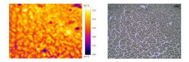
Figure 27. Thermographical image of the digestate being dried inside the greenhouse solar dryer (3<sup>rd</sup> August 2020).
