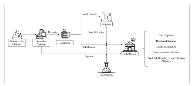
Figure 9. Digestate treatment line to produce dried organic fertilizer.
