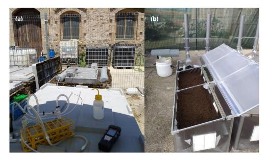
Figure 12. (a) Gas emission sampling during the storage of precision feeding manure and (b) Pilot scale greenhouse solar dryer.
