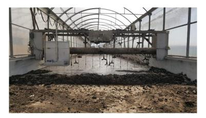
Figure 26. Greenhouse solar dryer and turning machine in the semi-industrial installation.
