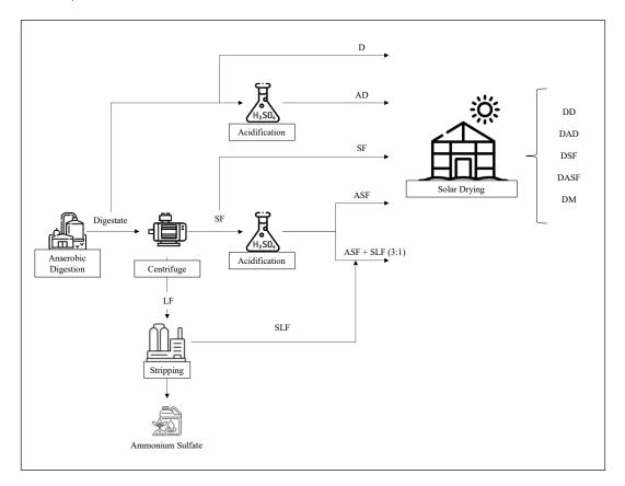
**Figure 25.** Diagram with all the digestate-derived fertilizers produced. Abbreviations: D, digestate; AD, acidified digestate; C, centrifuge; SF, solid fraction of digestate; LF, liquid fraction of digestate; ASF, acidified solid fraction; SLF, poor-nitrogen stream after LF stripping process; DD, dried digestate; DAD, dried acidified digestate; DSF, dried solid fraction; DASF, dried acidified solid fraction; DM, dried mixture of ASF and SLF.
