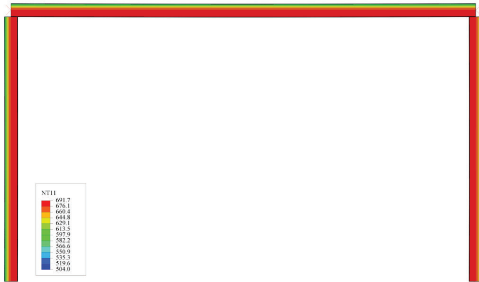
Figure 3.1. Temperature field [°C] of a stainless steel frame subjected to fire in its interior faces after 20 minutes.
