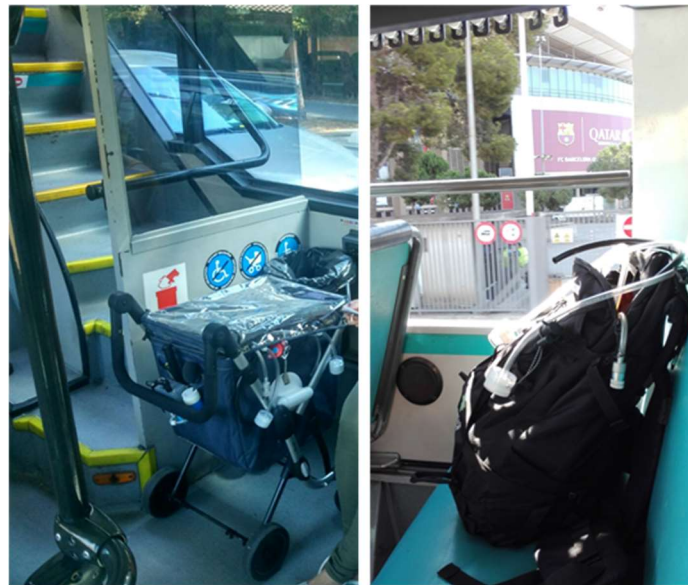
Figure 2.9. The sampling equipment inside tourist bus. In the left, the trolley that went in the lower floor, and in the right, the bag that went in the upper floor.
