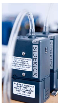
Figure 2.11. The cartridge and the pump used to measure VOCs inside buses.
