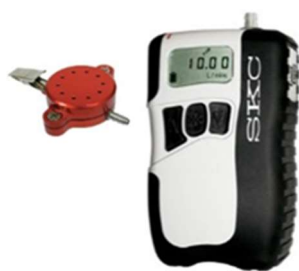
Figure 2.10. PEM and SKC pump used to sample PM_{2.5} fraction for chemical analysis.
