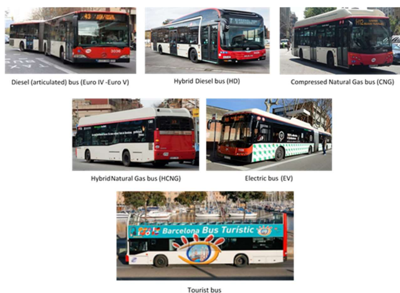
Figure 2.2. Different fuel/engine type buses from the fleet of TMB and the tourist buses.
