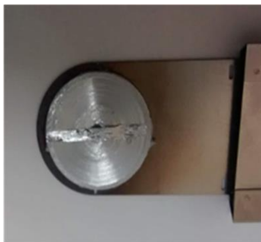
Figure 2.3 (a) BL04-MSPD (Material science and powder diffraction Beamline setup). (b) Linkam holder with the Al disc and the attached ribbons.
