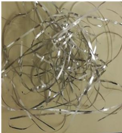
Figure 2.1 (a) Arc melter device, (b) scheme of the melt spinner, (c) ribbons produced by melt spinning.
