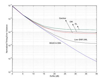
Figure 6.5: Normalized timing variance for the low-SNR ML and GML estimators as well as the EL (Early&Late), OM (Oerder&Meyr) and Gardner's symbol sychronizers. The simulation parameters are; 16-QAM, roll-off 0.25,  $N_{ss}=2$  ( $N_{ss}=4$  for the Oerder&Meyr),  $M = 2N_{ss}$  and,  $B_n = 5 \cdot 10^{-3}$ . The shaping pulse and the associated matched filter are truncated at  $\pm 5T$ .
