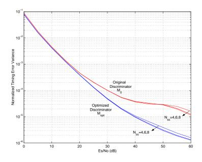
Figure 6.3: Timing error variance with and without loop optimization for  $N_{ss}$  equal to 4, 6 and 8 in case of the QPSK modulation with roll-off 0.1 and M=4.
