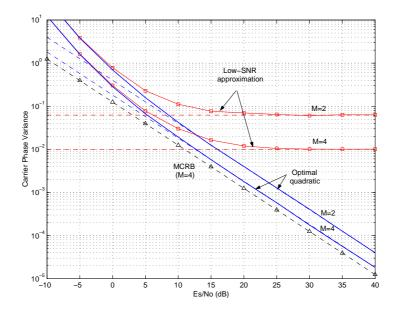
Figure 6.13: Carrier phase variance as a function of the SNR for the MSK modulation with  $N_{ss} = 2$ . Dotted lines correspond to the high-SNR bounds computed in Sections 6.2.3 and 6.2.5.
