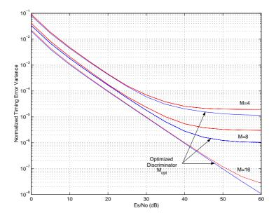
Figure 6.2: Timing error variance with and without loop optimization for different number of samples M in case of the QPSK modulation with roll-off 0.1 and  $N_{ss} = 2$ . The same curves are obtained for QAM and MPSK.
