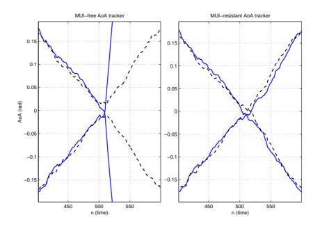
Figure 6.24: AoA tracking of two users whose trajectories cross at time instant n=500. The output of the MUI-free and MUI-resistant trackers is plotted on the left and right hand side, respectively. Two simulations are run with two different outcomes for the MUI-free tracker: tracking is lost (solid line) or the two sources are interchanged (dashed line). The signal SNR is fixed to 10 dB in both cases.
