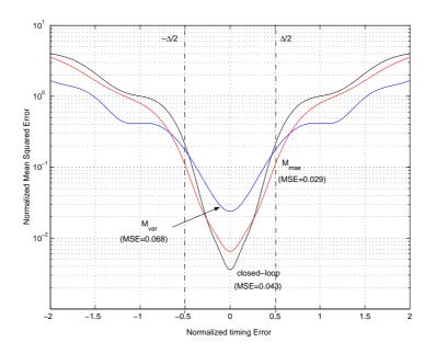
Figure 6.7: Normalized timing MSE for the MMSE, minimum variance and closed-loop secondorder estimators for K = 4 and Es/No=10dB. The average MSE for the three estimators is included inside round brackets.
