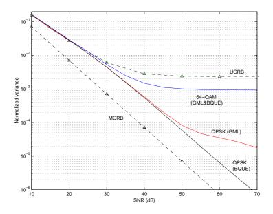
Figure 6.22: Comparison of the BQUE and GML estimators when the channel amplitude is estimated too and the transmitted symbols are QPSK, 64-QAM or, Gaussian distributed for a roll-off factor equal to 1.
