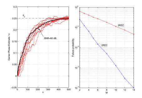
Figure 6.15: On the left side, 10 acquisitions for the 3REC modulation with  $N_{ss} = 2$  and M = 2. The SNR was set to 20 dB and the loop step-size fixed to  $\mu = 0.01$ . On the right-hand side, the probability of failure for 2REC and 3REC with  $N_{ss} = 2$  and  $\sigma_w^2 = 0$ .
