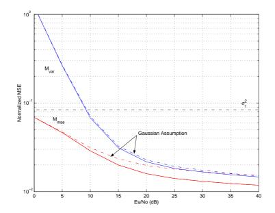
Figure 6.12: Normalized timing MSE for the MMSE  $(M_{mse})$  and minimum variance  $(M_{var})$  second-order estimators for the 16-QAM modulation when K = 4 and  $\Delta = 1$ . The suboptimal estimators deduced under the Gaussian assumption are also plotted.
