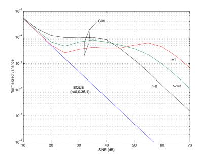
Figure 6.23: Comparison of the BQUE and GML estimators if the channel is multiplicative using different values of the roll-off factor.
