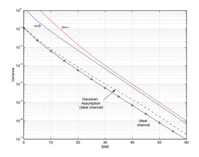
Figure 6.17: TOA estimation variance as a function of the SNR for MPSK symbols. The simulation parameters are  $N_{ss} = 4$  and M = 8. The transmitted pulse is a square-root raised cosine truncated at  $\pm 4T$  (100% roll-off).
