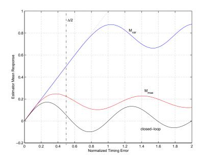
Figure 6.8: Estimation mean response for the MSE for the MMSE, minimum variance and closed-loop second-order estimators for K = 4 and Es/No=10dB.
