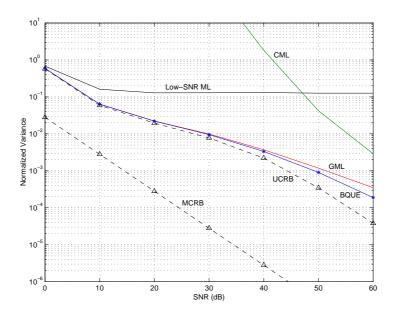
Figure 6.21: Performance of the second-order ML-based estimators (Low-SNR approximation, Conditional ML and Gausian ML) and the optimal solution provided in Chapter 4. The simulation parameters are r = 0.35,  $\mu = 0.02$  ( $B_n = 5 \cdot 10^{-3}$ ).
