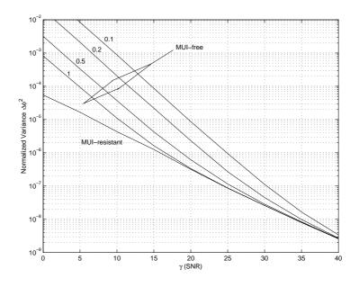
Figure 6.27: Normalized variance as a function of the SNR for the MUI-free and MUI-resistant AoA trackers when the sources are separated 0.1, 0.2, 0.5 or 1 as indicated for each curve. The tracker loop bandwidth is set to  $B_n = 1.25 \cdot 10^{-3}$ .
