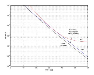
Figure 6.19: TOA estimation variance as a function of the SNR for the 2REC modulation. The simulation parameters are  $N_{ss} = 4$  and M = 8.
