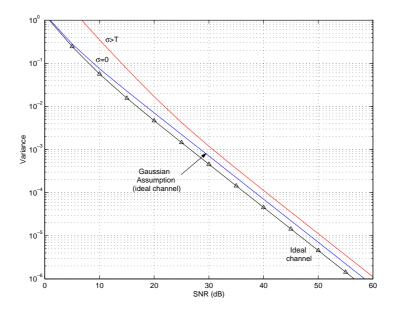
Figure 6.18: TOA estimation variance as a function of the SNR for MSK symbols. The simulation parameters are  $N_{ss} = 4$  and M = 8.
