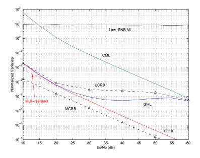
Figure 6.26: Steady-state variance of the AoA tracker for two sources located at  $\pm 0.5$  degrees from the broadside. The loop-bandwidth is set to  $B_n = 1.65 \cdot 10^{-4}$  and the MUI-free estimator is simulated.
