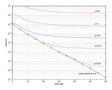
Figure 6.16: TOA estimation variance as a function of the SNR for 16-QAM symbols. The simulation parameters are  $N_{ss} = 4$  and M = 8. The transmitted pulse is a square-root raised cosine truncated at  $\pm 4T$  (100% roll-off).
