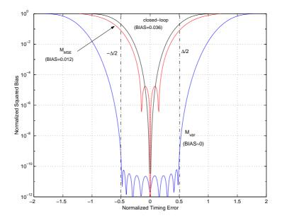
Figure 6.9: Normalized timing squared bias for the MMSE, minimum variance and closed-loop second-order estimators for K = 4 and Es/No=10dB. The average BIAS for the three estimators is included inside round brackets.
