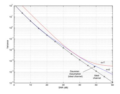
Figure 6.20: TOA estimation variance as a function of the SNR for the 3REC modulation. The simulation parameters are  $N_{ss} = 4$  and M = 8.
