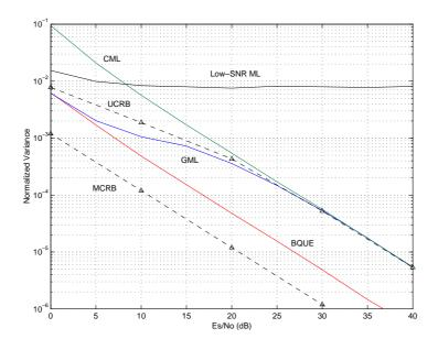
Figure 6.25: Steady-state variance of the AoA tracker for two sources located at  $\pm 5$  degrees from the broadside. The loop-bandwidth is set to  $B_n = 1.25 \cdot 10^{-3}$  and the MUI-free estimator is simulated.
