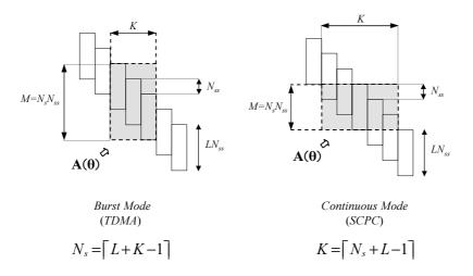
Figure 6.1: Structure of the transfer matrix  $\mathbf{A}(\boldsymbol{\theta})$  in a burst or continuous transmission.
