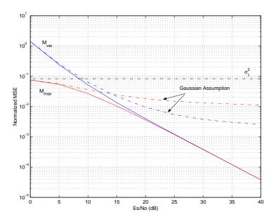
Figure 6.11: Normalized timing MSE for the MMSE  $(M_{mse})$  and minimum variance  $(M_{var})$  second-order estimators for the MSK modulation when K = 4 and  $\Delta = 1$ . The suboptimal estimators deduced under the Gaussian assumption are also plotted.
