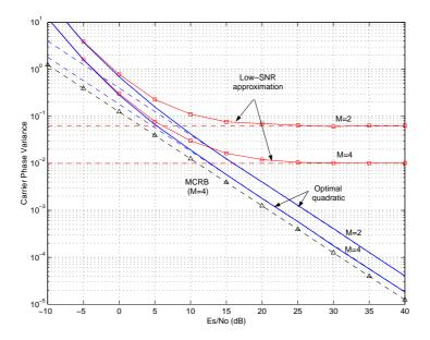
Figure 6.14: Carrier phase variance as a function of the SNR for the 3REC modulation with  $N_{ss} = 4$ .
