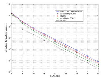
Figure 6.6: Normalized timing variance for the ML-based estimators for the MSK modulation with  $N_{ss}=2$ , M=4 and,  $B_n = 5 \cdot 10^{-3}$ .
