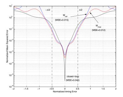
Figure 6.10: Normalized timing MSE for the MMSE, minimum variance and closed-loop secondorder estimators for K = 4 and Es/No=40dB. The average MSE for the three estimators is included inside round brackets.
