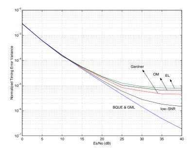
Figure 6.4: Normalized timing variance for the low-SNR ML and GML estimators as well as the EL (Early&Late), OM (Oerder&Meyr) and Gardner's symbol sychronizers. The simulation parameters are; 16-QAM, roll-off 0.75,  $N_{ss}=2$  ( $N_{ss}=4$  for the Oerder&Meyr),  $M = 2N_{ss}$  and,  $B_n = 5 \cdot 10^{-3}$ . The shaping pulse and the associated matched filter are truncated at  $\pm 5T$ .
