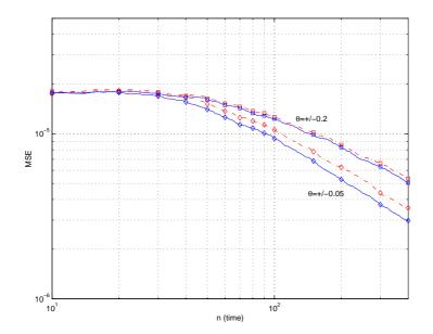
Figure 5.6: Estimation MSE as a function of time for the optimum and Gaussian QEKF (dashed) in the case of two MPSK-modulated signals received from  $\pm 0.2$  ( $\Box$ ) and  $\pm 0.05$  ( $\diamondsuit$ ) when  $R_u$  is set to zero at time n=20 and the SNR is equal to 10dB.
