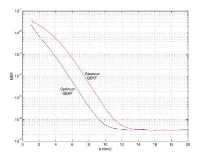
Figure 5.1: Estimation MSE as a function of time for the optimum and Gaussian QEKF in the case of a single static MPSK-modulated user with random DOA in the range  $\pm 0.4$  and SNR=40dB.
