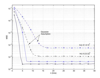
Figure 5.2: Estimation MSE as a function of time for the optimum and Gaussian QEKF in the case of two static MPSK-modulated users placed at  $\pm 0.2$ ,  $\pm 0.1$  and SNR=40dB.
