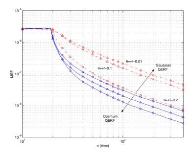
Figure 5.3: Estimation MSE as a function of time for the optimum and Gaussian QEKF (dashed) in the case of two static MPSK-modulated sources transmitting from  $\pm 0.2$  ( $\Box$ ),  $\pm 0.1$  ( $\triangle$ ) and,  $\pm 0.01$  ( $\diamondsuit$ ) when  $\mathbf{R}_u$  is set to zero at n=20. SNR=40dB.
