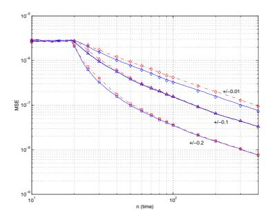
Figure 5.5: Estimation MSE as a function of time for the optimum and Gaussian QEKF (dashed) in the case of two 16-QAM modulated signals received from  $\pm 0.2$  ( $\Box$ ),  $\pm 0.1$  ( $\triangle$ ) and  $\pm 0.01$  ( $\diamondsuit$ ) when  $R_u$  is set to zero at time n=20. SNR=40dB.
