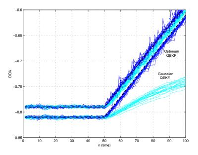
Figure 5.4: DOA Tracking of two close MPSK-modulated signals separated 0.02 using the optimum and Gaussian QEKF. SNR=40dB.
