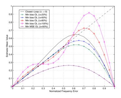
Figure 3.2: Estimator mean response for different values of  $\Delta$ . The simulation parameters are M=4,  $N_{ss}=2$ , Es/No=10dB.
