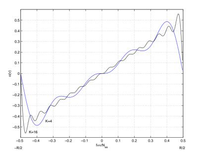
Figure 3.10: Mean value of the frequency estimator corresponding to the minimum bias solution for K=4 and 16.
