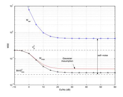
Figure 3.6: Normalized MSE for the MMSE and the minimum variance frequency estimators deduced in (3.25) and (3.30) for the MPSK modulation. The transmitted pulse is a square-root raised cosine with roll-off 0.75 truncated at  $\pm 5T$ . The corresponding estimators deduced under the Gaussian assumption are also plotted for comparison. The simulation parameters are M = 8,  $N_{ss} = 2$ , K = 13 and  $\Delta = 1.6$ .
