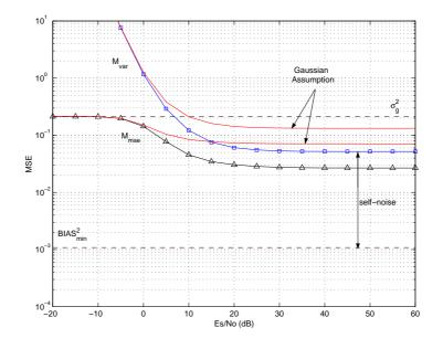
Figure 3.4: Normalized MSE for the MMSE and the minimum variance frequency estimators deduced in (3.25) and (3.30) for the MSK modulation. The corresponding estimators deduced under the Gaussian assumption are also plotted for comparison. The simulation parameters are M = 8,  $N_{ss} = 2$  and  $\Delta = 1.6$ .
