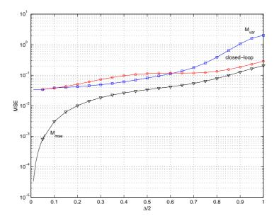
Figure 3.9: MSE as a function of  $\Delta$  for the MSK modulation. The simulation parameters are Es/No=10dB, M = 4 and  $N_{ss}=2$ .
