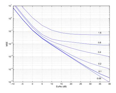
Figure 3.7: MSE corresponding to the minimum variance solution for different values of the parameter range  $\Delta$ =0.05, 0.1, 0.2, 0.4, 0.8 and 1.6. The received signal is MSK-modulated and M=8 samples are processed with N<sub>ss</sub>=2.
