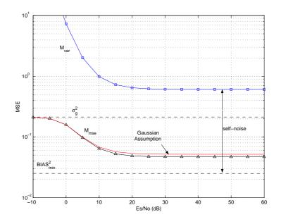
Figure 3.5: Normalized MSE for the MMSE and the minimum variance frequency estimators deduced in (3.25) and (3.30) for the 16-QAM modulation. The transmitted pulse is a square-root raised cosine with roll-off 0.75 truncated at  $\pm 5T$ . The corresponding estimators deduced under the Gaussian assumption are also plotted for comparison. The simulation parameters are M = 8,  $N_{ss} = 2$ , K = 13 and  $\Delta = 1.6$ .
