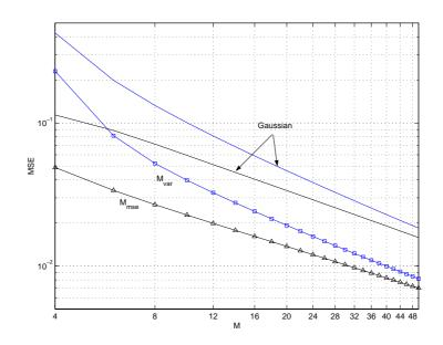
Figure 3.8: Normalized MSE for the MMSE and the minimum variance frequency estimators deduced in (3.25) and (3.30). The modulation is MSK, Es/No=40dB,  $N_{ss} = 2$  and  $\Delta = 1.6$ .
