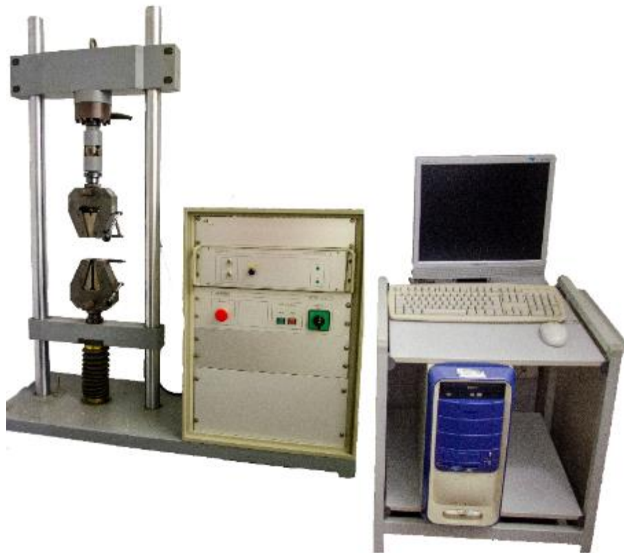
Figure 11: Tensile testing machine for adhesion testing.
