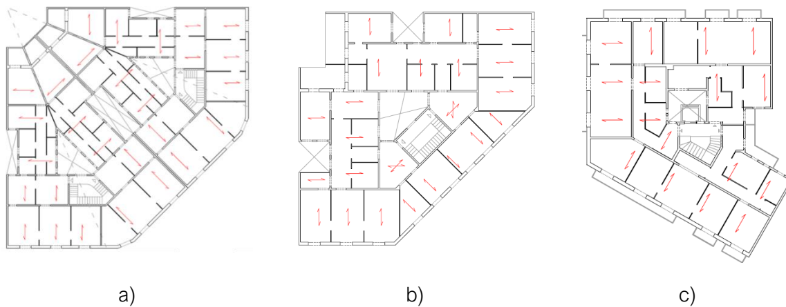
Figure 3.39 - Chamfer buildings' geometrical configurations located at each corner of the urban block: a) Chamfer buildings with radial structural distribution of the walls parallel to the façade; b) Chamfer buildings geometrically composed of two parts: "L" shape and a triangular part; c) Corner buildings that do not represent the typical chamfer characteristics (Cornadó Bardón, 2015).
