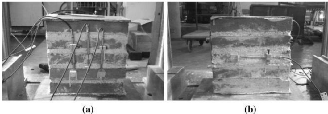
Figure 3.62 - Masonry prisms with a typical layout of LVDTs: a) vertical layout for displacement measurement in the unit and the composite and b) horizontal displacement for measurement of the Poisson's ratio (Drougkas et al., 2016).
