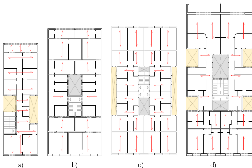
Figure 4.4 - Position and number of interior (in grey) and lateral (in yellow) patios in different plan configurations: a) building with lateral patios; b) building with interior central patio; c) building with interior patios near the central staircase and lateral patios on each side of the longitudinal masonry wall; d) buildings with interior central patios and two or more lateral patios on each side of the longitudinal masonry wall (adapted from Cornadó Bardón 2015).
