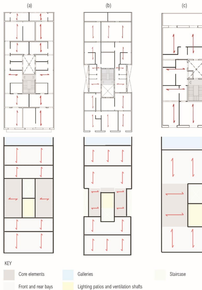
Figure 4.14 - Examples of structural plan distributions of the typical band buildings of the Eixample district composed of central part with the staircase and the lighting and ventilation patios, the front and rear bays, and the galleries at the back façade: a) band building with central stairwell and light patio; b) band building with central stairwell and lateral semi-patios, and c) narrow band building with lateral stairwell and lateral lighting patio (adapted from Cornadó Bardón 2015).
