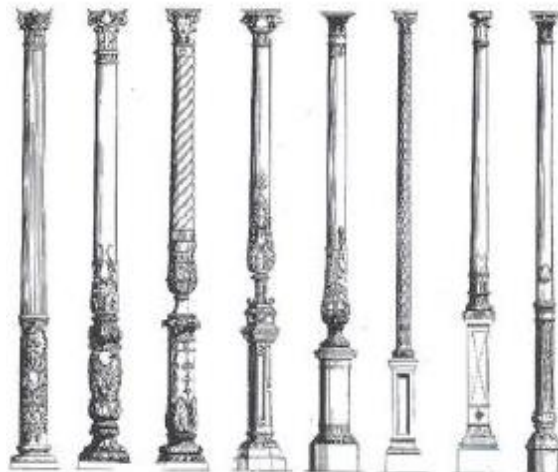
Figure 3.32 - Decorated cast-iron pillars in the existing historical buildings in Eixample district (Rigalt i Fariols, 1857).
