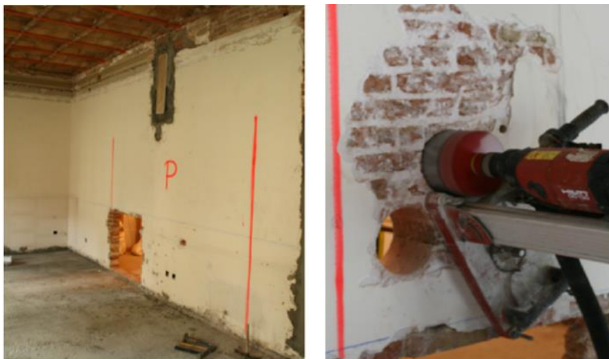
Figure 3.58 - Interior masonry wall to be tested from an existing Eixample building (left) and in-situ core drilling (right) (Segura et al., 2019).
