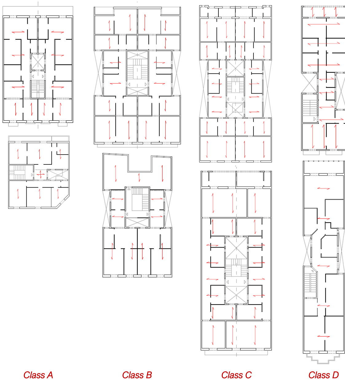
Figure 7.8 - Definition of vulnerability classes for Parameter 4 "Plan configuration" with examples of existing buildings plan configurations (adapted from Cornadó Bardón 2015).
