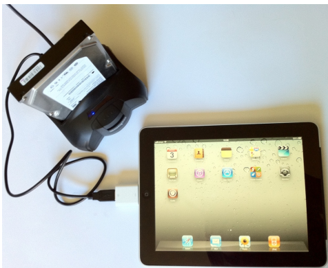
Figure 2. iPad connection to external hard drive via Camera Connection Kit.
