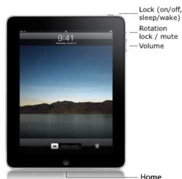
Figure 1. iPad button configuration (iOS 4 and higher).
