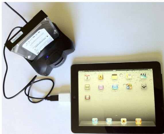
Fig. 2. iPad connection to an external hard drive via Camera Connection Kit.
