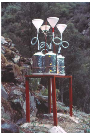
Figure 3.8. Image of the bulk deposition sampler at La Castanya.
