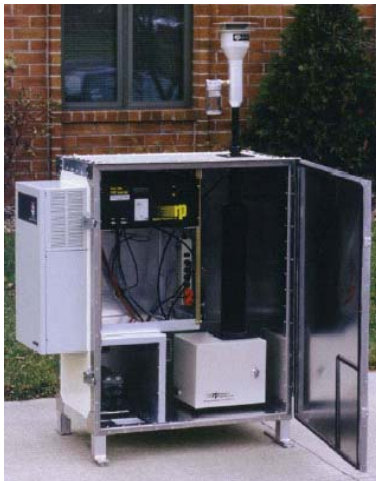
Figure 3.6. Image and scheme of the typical installation of a Rupprecht & Patashnick TEOM instrument model 1400a (from http://www.rpco.com/ ).
