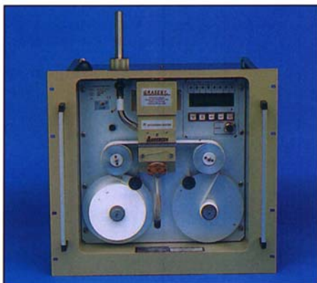
Figure 3.7. Image and scheme of an Andersen \beta -attenuation instrument model FH62I-N (from http://www.esm-online.de/andersen/ ).
