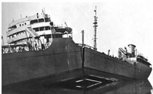
Figure 1.1: Ship failure – Callister (1997).
