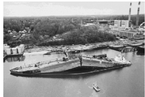
Figure 1.1: Ship failure – Callister (1997).
