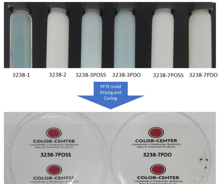
Figure 6. Appearance of the synthesized WPUD (top) and casted films (bottom) from two of the polyurethane-urea dispersions (3238-7POSS and 3238-7PDO).
