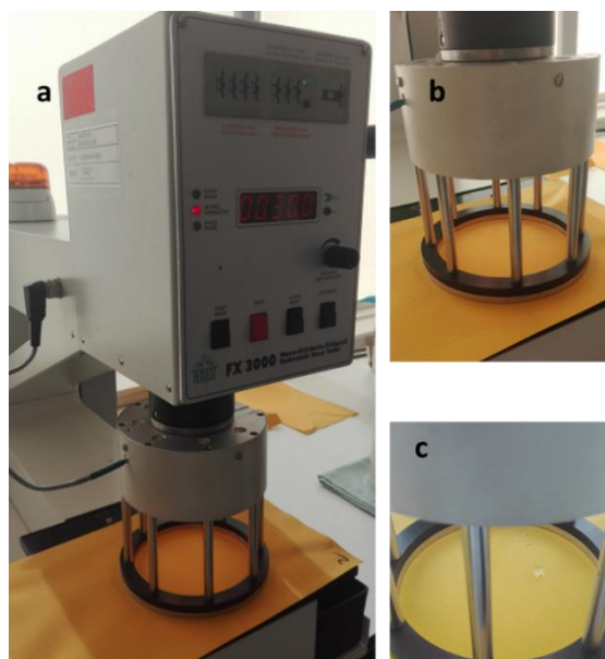
Figure 33. Device used to the measurement of resistance to water penetration -water column or hydrostatic pressure test-. (a) General view, (b) pressure unit, (c) the fabric begins to yield to the water pressure, as denoted by the appearance of water droplets.
