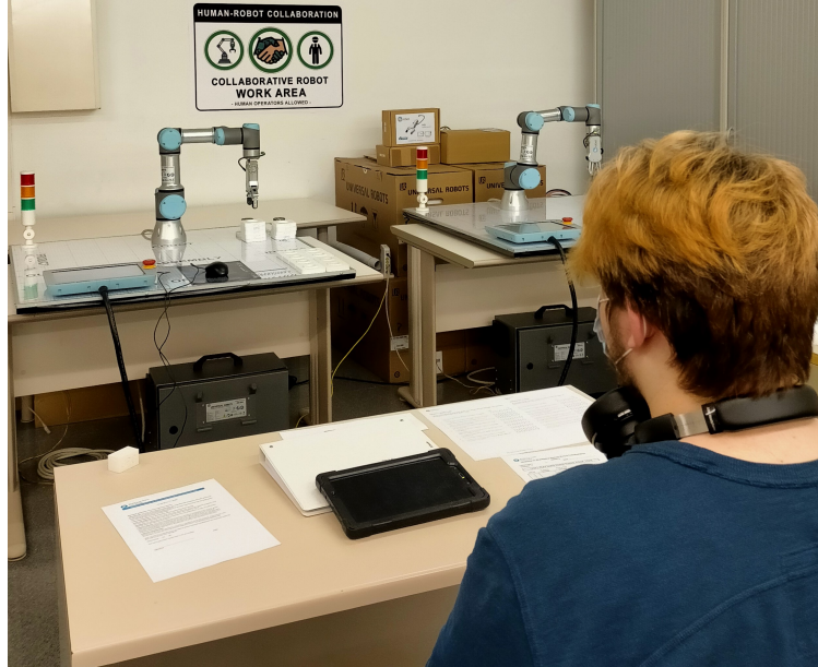
Figure 3.12: Laboratory resources: the main task developed on a tablet and the secondary collaborative task of assembly with the robot on the left in the background
