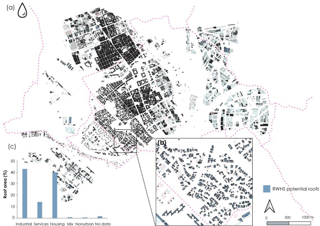
Figure 5.9. (a) Potential rooftops for integrating RWHS over the study area. (b) Details of identified potential roofs in housing and services buildings. (c) Potential roofs identified to integrate RWHS and their distribution by land use. (d) Water self-sufficiency for laundry, showering, toilet flushing, cleaning, and irrigation (no agricultural) uses.
