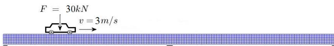
Figure 4. Loading in the form of a moving concentrated vertical force (force: F=30\text{kN} , speed: v = 3\text{m/s} ).
