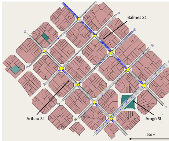
Figure 4.1: Screenshot of the Aimsun Next microscopic DTA simulation showing the working domain, where the three major streets are pointed: Aribau St on the left (representation of normal flow), Aragó St on the right (representation of free flow) and Balmes St on top (representation of congested flow). Simulated individual vehicles in each street are represented in blue.
