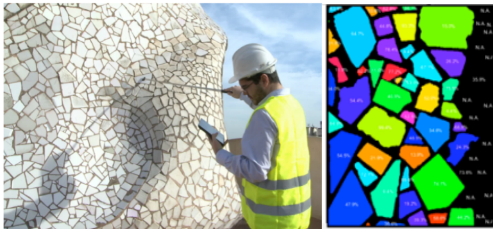
Figure 22. System to detect adherence of tiles, developed in the PDP course.
