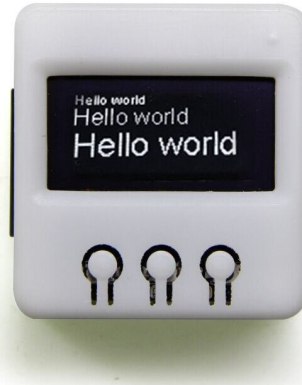
(b) Prototype of a home device in a 3D-printed case.
