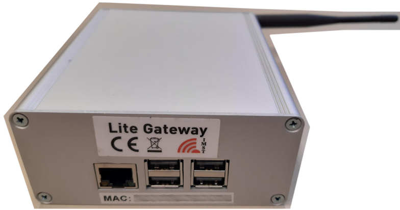
Figure 2.4: An indoor IMST LoRaWAN gateway based on a Raspberry Pi computer and an iC880A concentrator.
