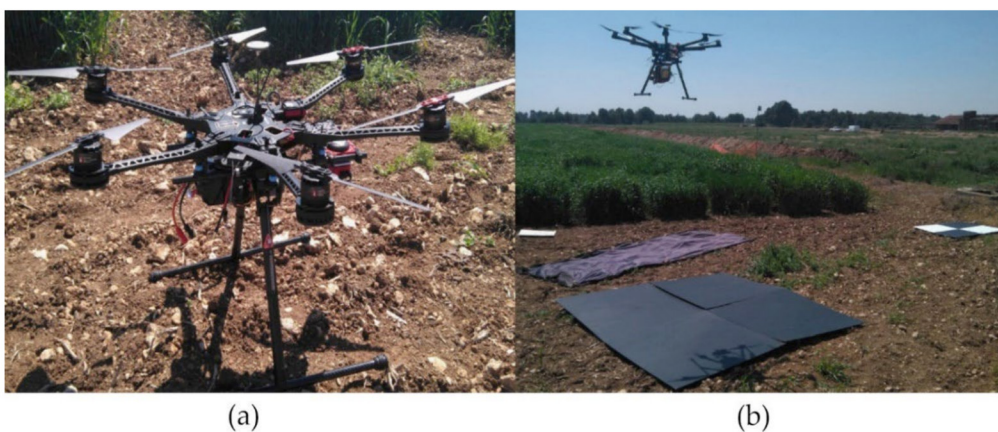
Figure 2. (a) Unmanned aerial vehicle (UAV) Hexacopter DJI S800 EVO used to collect the multispectral images of the experimental plots; (b) reference targets used for the geometric and radiometric calibrations.
