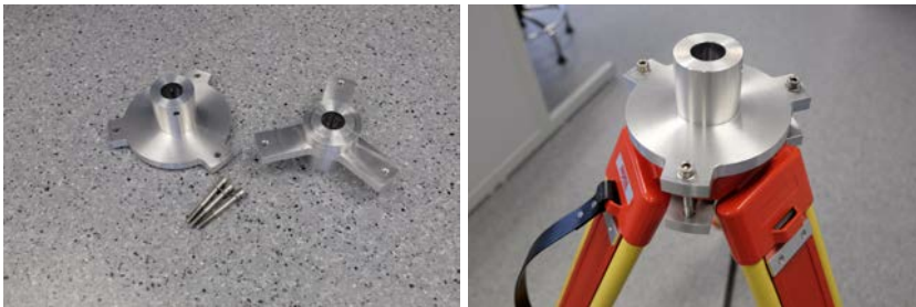
Figure A.3: Top baseplate (left), and bottom baseplate (right), and baseplate screws. In the picture they are shown in the correct mounting orientation. The right image shows the baseplates attached to the top of the tripod.
