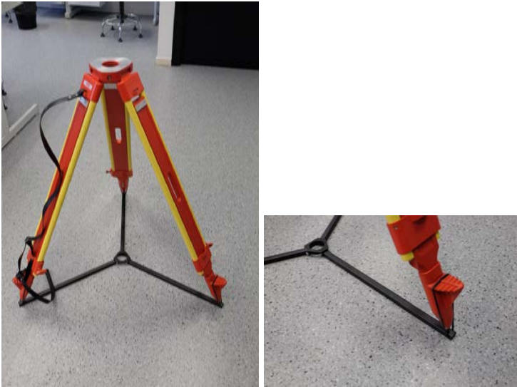
Figure A.2: Mounted tripod, and tripod legs inserted into the tripod base.
