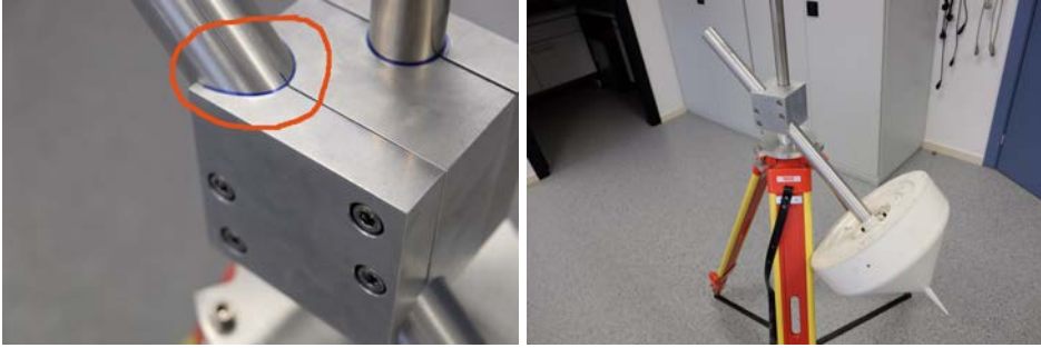
Figure A.6: The blue line at the 45 degrees down-looking pole shall be as in the picture.
