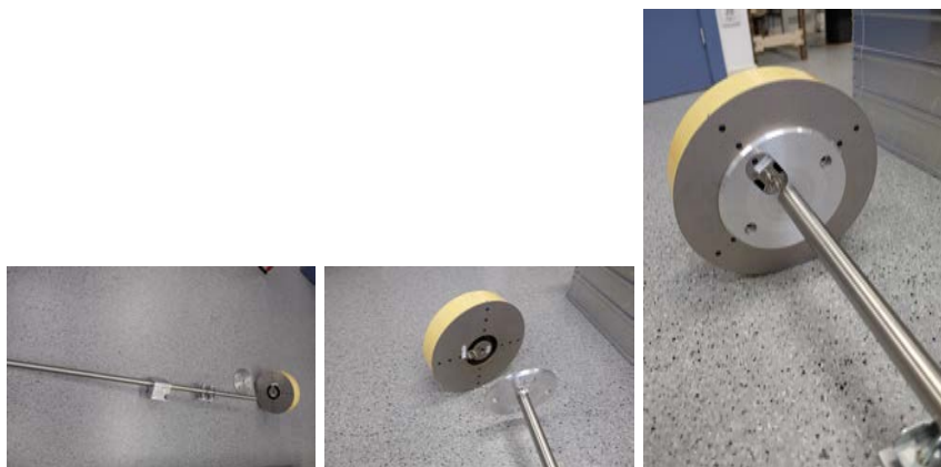
Figure A.4: Up-looking antenna mounted at the top of the pole.
