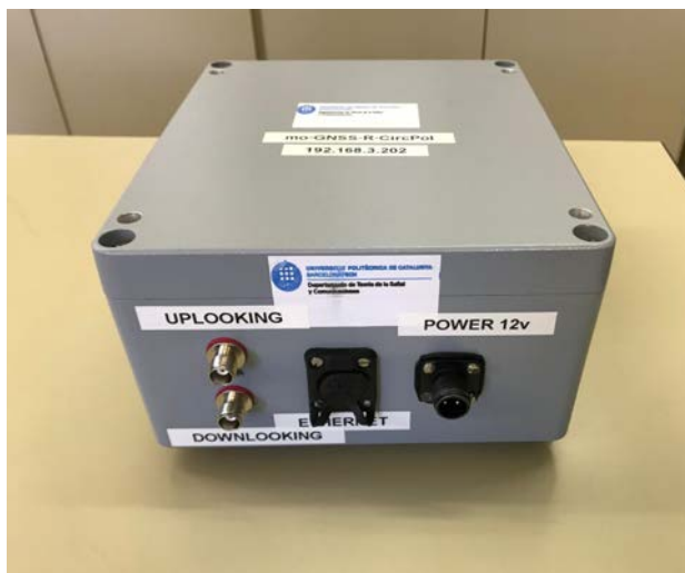
Figure 7.2: PYCARO-2 instrument enclosed inside its aluminum box.
