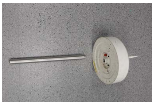
Figure A.5: 45 degrees down-looking antenna shall be screwed to its pole.
