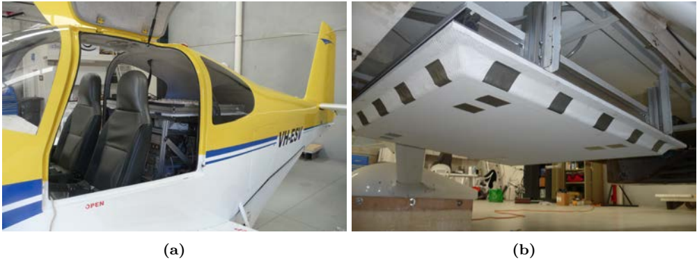
Figure 4.1: (a) (MIR) instrument and up-looking array mounted inside the airplane, and (b) down-looking array covered with a radome hanging from the airplane's fuselage [128].
