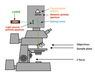
Figure 16. Confocal microscope scheme
