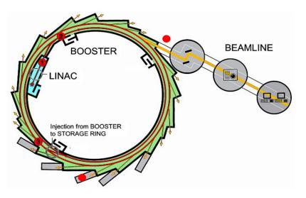
Figure 22. ALBA synchrotron scheme. 1. LINAC, 2. Booster ring, 3. Storage ring 4. Beamline [107]
