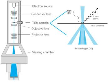
Figure 15. TEM schematic representation. In the right part of the image, a representation of all the possible trajectories of the electrons resulting of the interactions with the sample; in brackets, the detector for measurement.
