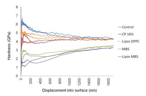
Figure 3. Continuous stiffness measurement for the different treatments tested
