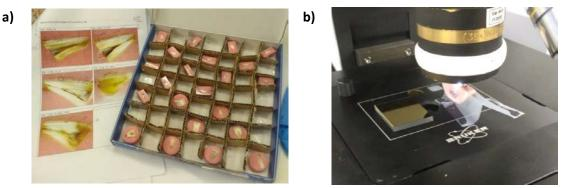
Figure 21. a) Tooth samples with specular polishing. b) FTIR microscope objective pointing on the sample; at its side, a golden mirror (perfect mirror) used as a reference to acquire the reflectance baseline.
