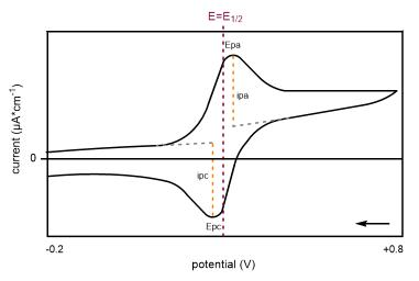
Figure 14. Typical voltammogram in the IUPAC convention
