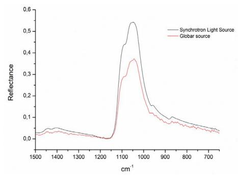
Figure 23. Specular reflectance spectra from a point in the enamel. Red: spectra obtained with globar internal source, at 10x10 μ aperture and 256 scans. Blue: spectra obtained with synchrotron light source, at 5x15 μm aperture and 256 scans. Data obtained in MIRAS beamline (ALBA synchrotron).
