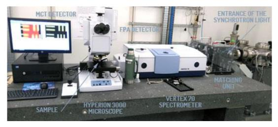
Figure 24. MIRAS beamline in ALBA Syncrotron (Source: https://www.cells.es/en/beamlines/bl01-miras)
