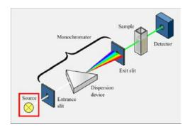
Figure 11. Spectrophotometer scheme
