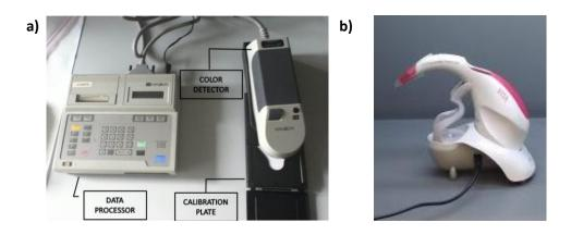
Figure 13. a) Minolta chroma meter CR-231 (equipment used in this work). b) Vita Easyshade Compact system, colorimeter adapted for its use in clinics
