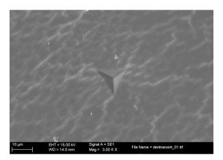
Figure 17. Scanning electron microscopy (SEM) image of a nanoindentation performed on the polished enamel of a bovine tooth
