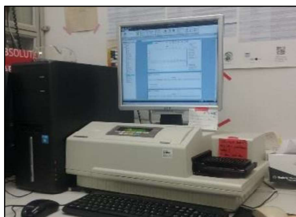
Figure 4.13. Microplate reader for total fluorescence measurements to determine cell number concentration in a biological sample.
