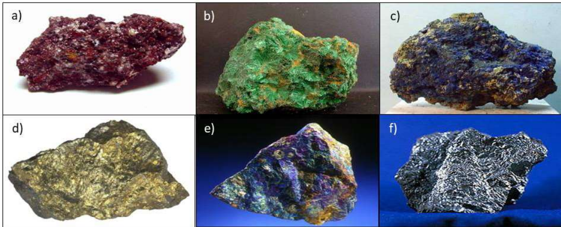
Figure 2.9. Pictures of the most common ores containing copper: a) cuprite; b) malachite; c) azurite; d) chalcocopyrite; e) bornite; and, f) chalcocite (Fundación integra 2014; Mundo mineral 2013).
