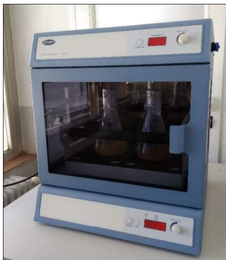
Figure 4.2. Incubator used for the cultivation of Acidithiobacillus ferrooxidans in batch conditions.
