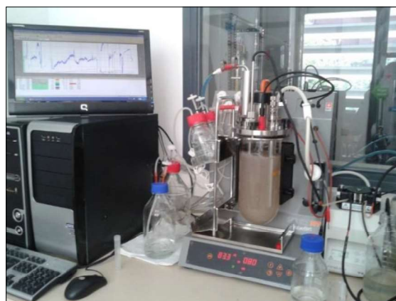
Figure 4.1. Fermenter used for the cultivation of the mixed microbial consortium.
