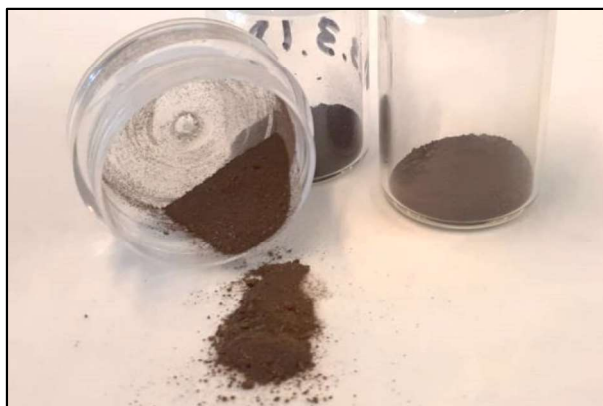
Figure 10.4. Metallic copper obtained as a fine brown powder by cementation.
