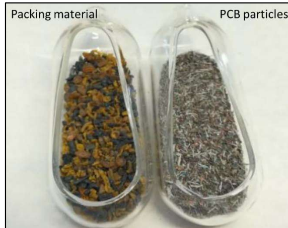
Figure 9.11. Packing material and PCB particles used in the experiment in which the plastic structure of the mobile phones was evaluated as a packing material in the column reactor.
