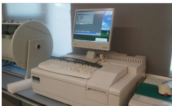
Figure 4.12. UV-Vis spectrophotometry to analyse iron (II) and iron (III) in liquid samples.
