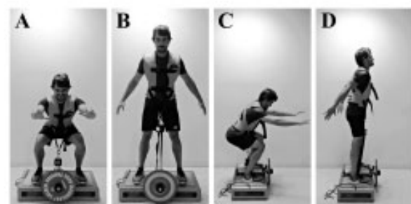
FIGURE 1 | Concentric–eccentric bilateral half-squats performed on a “YoYo squat” inertial flywheel device; anterior view (A,B), lateral view (C,D). (A,C) Bottom position of the exercise and transition between the eccentric and the concentric phases. (B,D) Top position of the exercise and transition between the concentric and the eccentric phases. The vest is attached to a strap wound on the flywheel axis. As resistance is the moment of inertia of the flywheel, the force applied during the concentric phase to unwind the strap determines the force needed during the eccentric phase (as the strap rewinds) to impede the spin of the axis.
