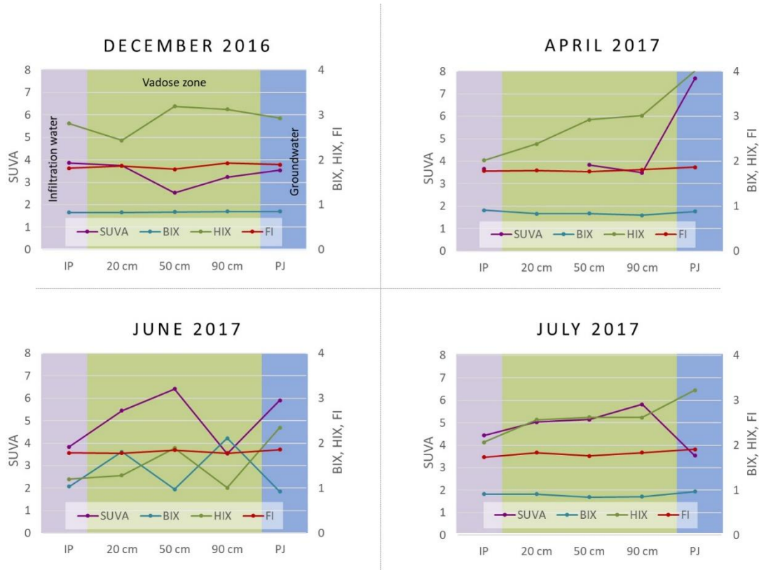
Figure 4.9 Evolution of fluorescence indices (SUVA, BIX, HIX, and FI) of water samples in the Castellbisbal MAR system for four different sampling campaigns
