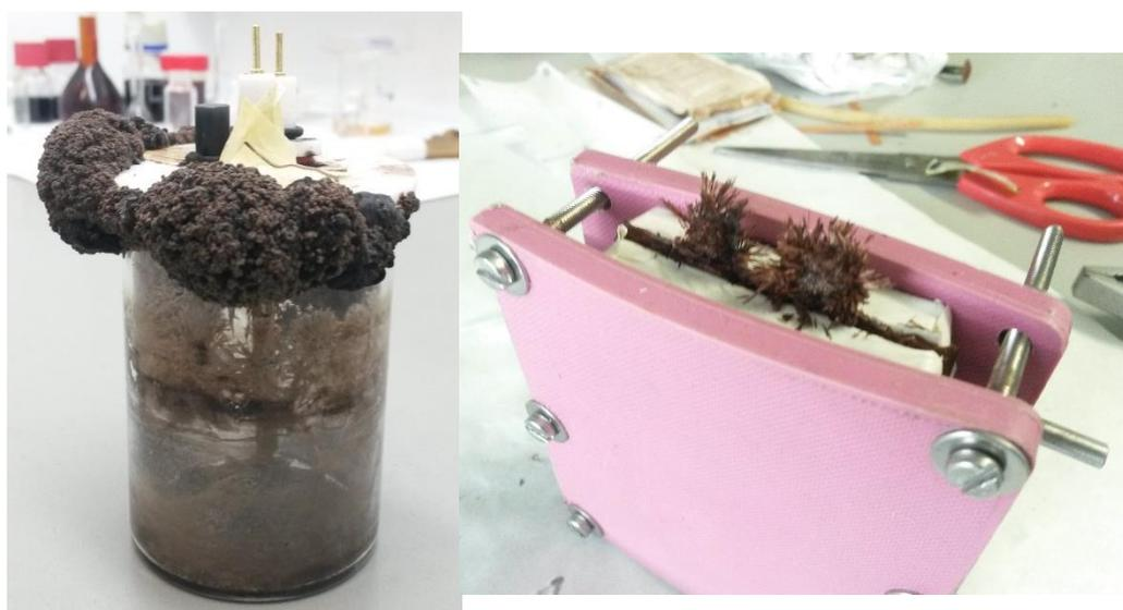
Fig. 13 Digital pictures of quinone crystallization outside of different electrochemical cells.
