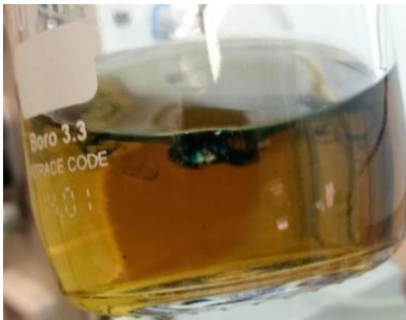
*Fig.9 Metal lithium on a 0.01M MBQ solution on CH<sub>3</sub>CN. The green layer formed on the surface of metallic lithium is apparent in this photograph.*
