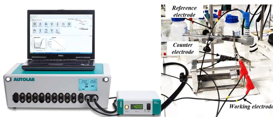
Fig. 6.2. Three-electrode electrochemical cell system.
