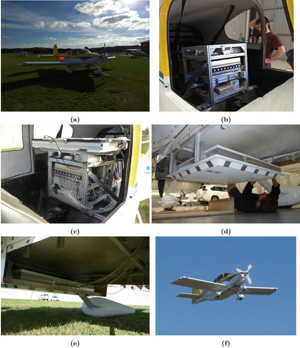
Figure 11.3: Photos of the MIR assembly in the aircraft: (a) side view of the aircraft, (b) MIR rackmount inside the aircraft, (c) up-looking array placed over the rackmount, (d) down-looking array being mounted on the aircraft belly, (e) view of the cables from the down-looking array to the rackmount, and (f) aircraft flight showing the down-looking array.
