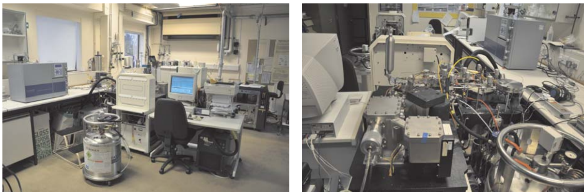
Figure 3.6. Images of the carbon isotope analyser used at the NERC Isotope Geosciences Laboratory for the extraction of carbon (as \text{CO}_2 ) from biogenic silica and for analysis by means of an Optima mass spectrometer.
