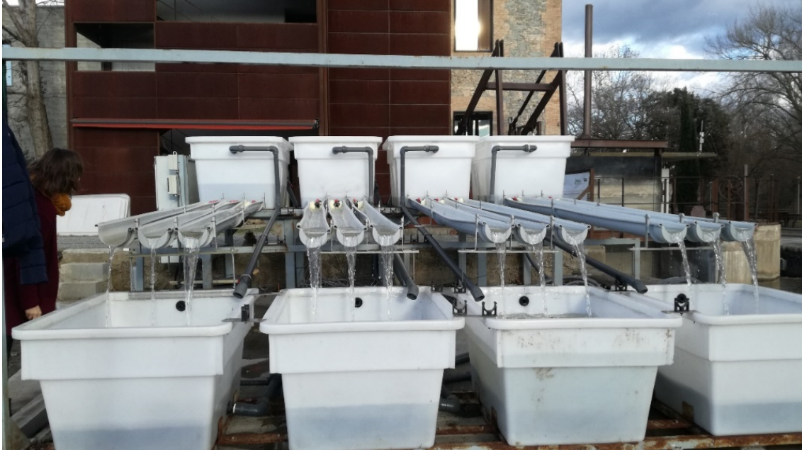
Figure 1.6. Experimental flumes at the Ter River Museum (Manlleu, NE Spain) used in this Thesis to evaluate the effect of water flow and light availability on biofilm community composition and geosmin production. March 19, 2018.
