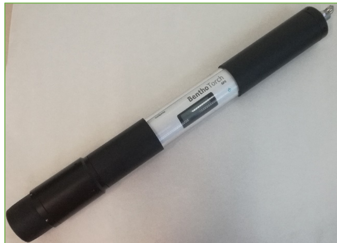
Figure 3.14. BenthosTorch (bbe Moldaenke, Schwentineta, DK) using in the in situ biofilm community measurements performed in the different experiments done in this Thesis.
