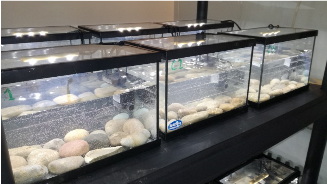
Figure 1.5. Microcosms (aquariums) at BETA Technological Center (Vic, Spain) used in this Thesis to evaluate the effect of nutrient concentration and N:P ratio on biofilm community development and geosmin production. March 18, 2019.
