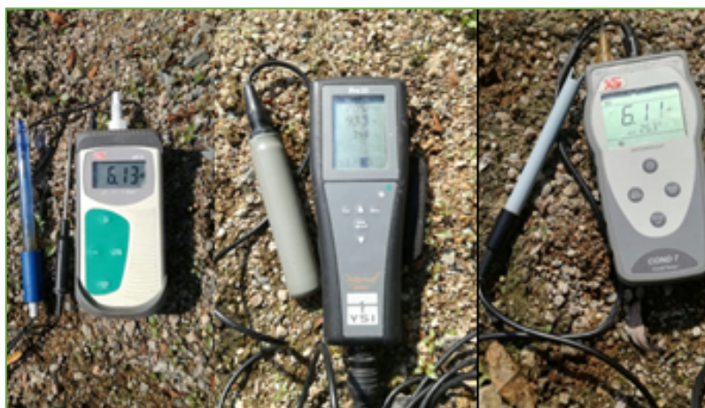
Figure 3.11. From the left to the right, portable probe for pH, oxygen and temperature and electrical conductivity.
