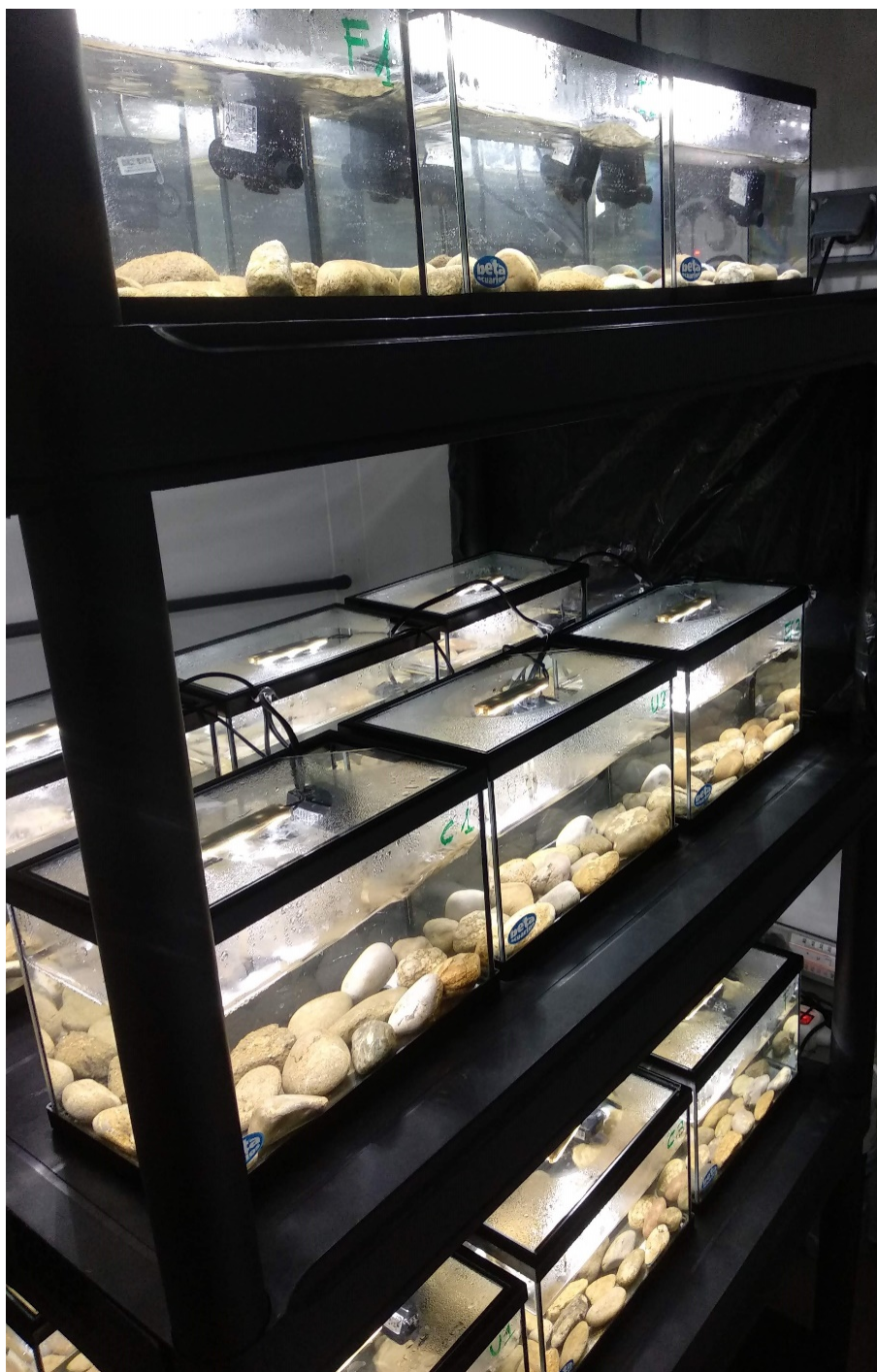
Figure 4.1. Microcosms (aquariums) used in this experiment to evaluate the effect of N:P ratio and nutrient concentration on biofilm community development and geosmin production and release. Laboratory of BETA Technological Center, Vic (Spain).
