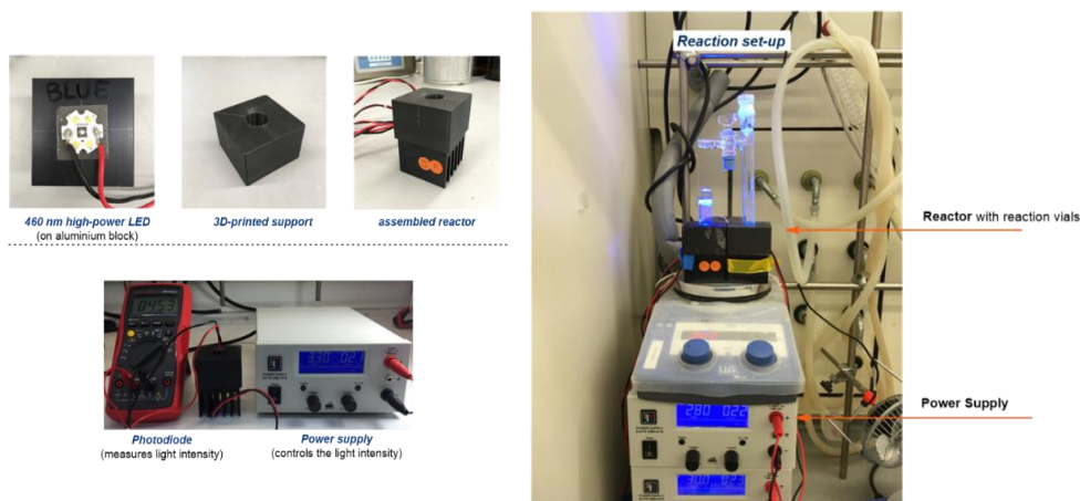
Figure S4.4. Detailed set-up and illumination system. The light source for illuminating the reaction vessel consisted of a 460 nm high-power single LED (OCU-440 UE420-X-1) purchased from OSA Opto Light.
