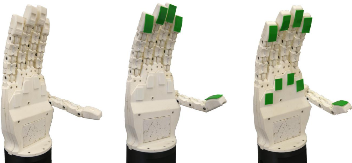
Figure 1. The three configurations of the ARMAR hand with different sets of friction pads; from left to right versions A1, A2 and A3.
