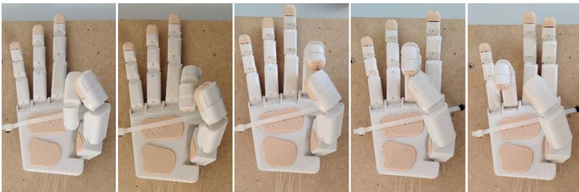
Figure 5. IMMA hand performing the Kapandji opposition test (KOT) in positions 1 (left) to 5 (right).
