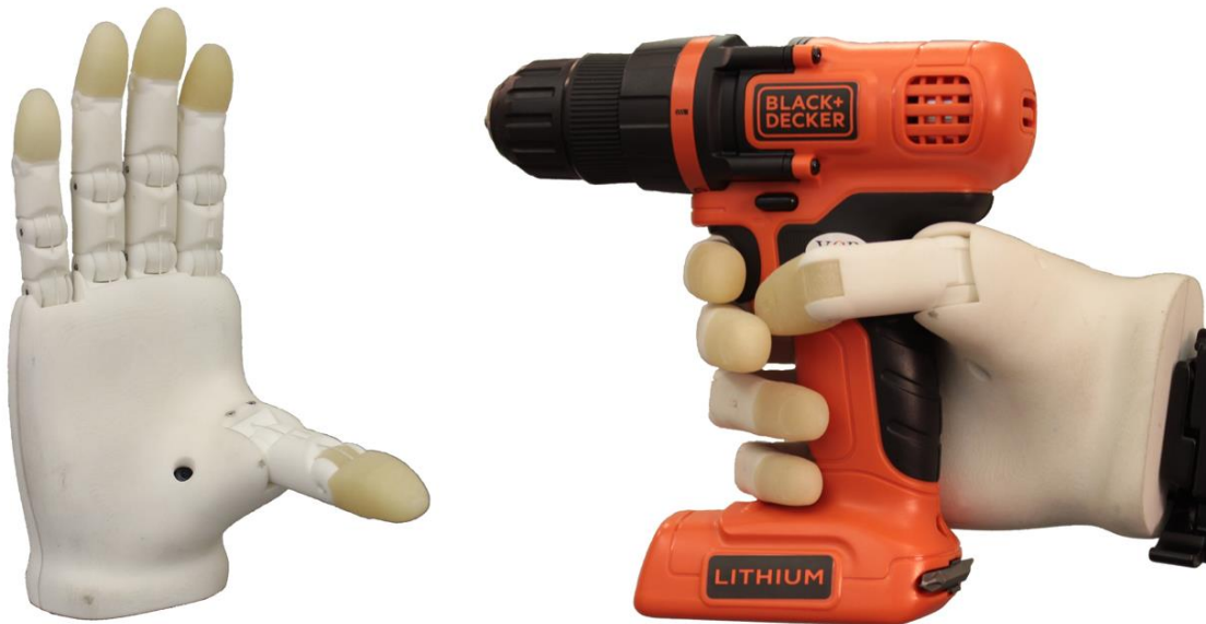
Figure 2. The final version of the KIT Prosthetic Hand (P2) fully opened (left) and while grasping the power drill (right).
