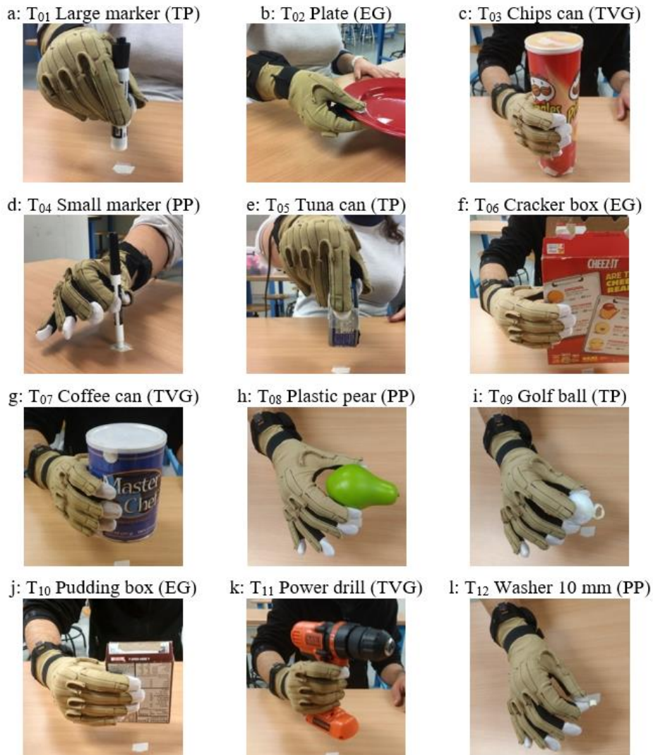
Figure 2. Grasping tasks of the experiment (a-l). T_g are the tasks ordered (g: indicates the order) followed by the object of the Yale-CMU-Berkeley Object and Model Set (Calli et al., 2015) to grasp and in brackets the grasp type to be performed in each task (TP: tripod pinch, EG: extension grip, TVG: transverse volar grip, PP: pulp pinch).
