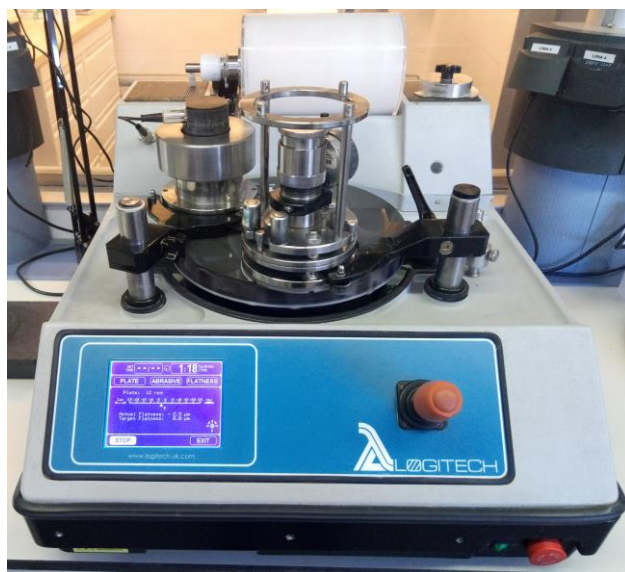
Figure 2.5. Logitech PM5 autopolisher during the lapping process.
