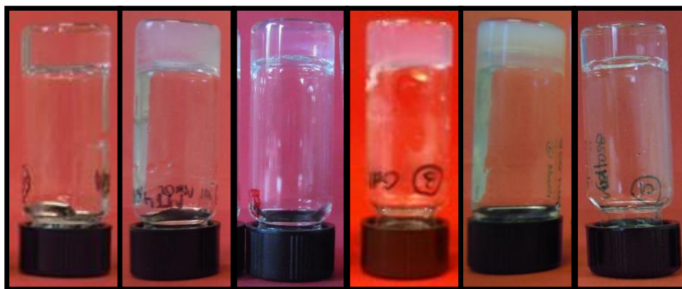
Figure 4.4 Macroscopic aspect of the hydrogels at their m.g.c. for compounds 1-6 (from left to right).
