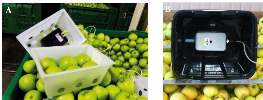
Figure 1.5 A) Harvestwatch (HA) sensor (Isolcell, Canada). B) Fruit Observer (FO) sensor (Besseling, The Netherlands).
