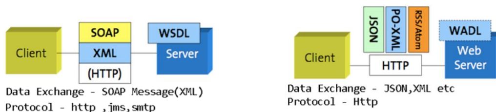
Figure 1.20: Web services architecture (a) versus REST services (b)
