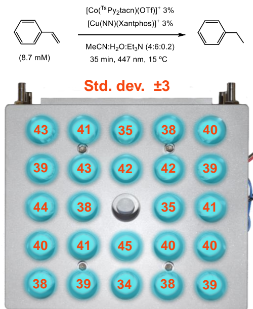
Figure A.VII.2. Reproducibility of the 24-well photoreactor in the photoreduction of styrene ( 13a ) as model substrate. Conditions A: Co-Cat (261 \mu M, 3% mol), PSCu (261 \mu M, 3% mol), 13a (16 \mu mol, 8 mM) in H 2 O:CH 3 CN:Et 3 N (6:4:0.2 mL) irradiation (447 nm) for 5h at 15 °C under N 2 . Yields determined by GC analysis after workup relative to a calibrated internal standard. Values were average of triplicates. Values are ethylbenzene ( 14a ) GC-FID yields.
