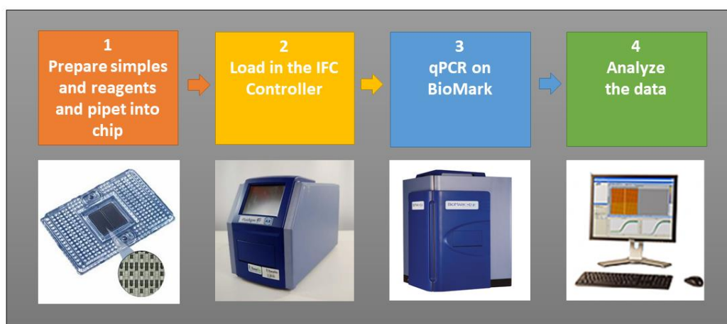
Figure 3. 1 Fluidigm BioMark system workflow. Figure adapted from www.Fluidigm.com .
