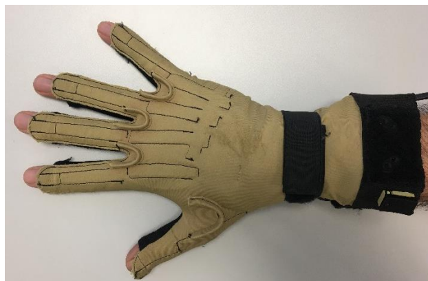
Figure 7.1 Cyberglove I device and the strap used for the wrist sensors
