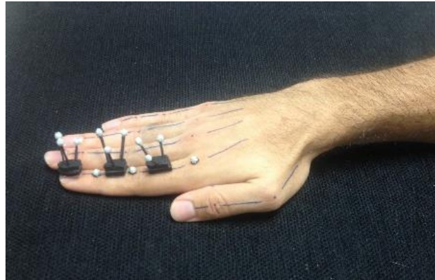
Figure 1.12 Reference posture with landmarks and tracking markers on the index finger
