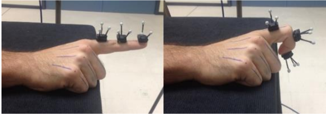
Figure 1.14. Movements recorded. (Left) Initial (and final) posture of the F/E movement for the index finger. (Right) Maximum flexion posture of the F/E movement for the index finger.
