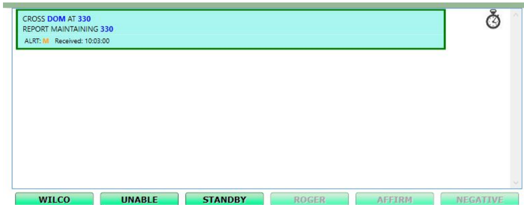
Figure 20: Only those hotkeys that would be valid replies appear enabled when the message to be answered is selected.
