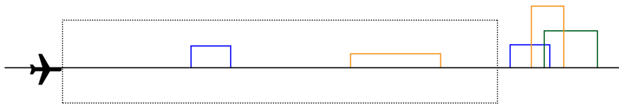
Figure 10: Workload forecast window. Conflicting overlaps will not try to be solved by the system until they do not enter in the time window being monitored.
